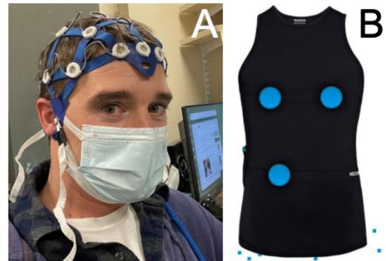
**Figure 1.** Example of microEEG device (A) and Hexoskin device (B).
